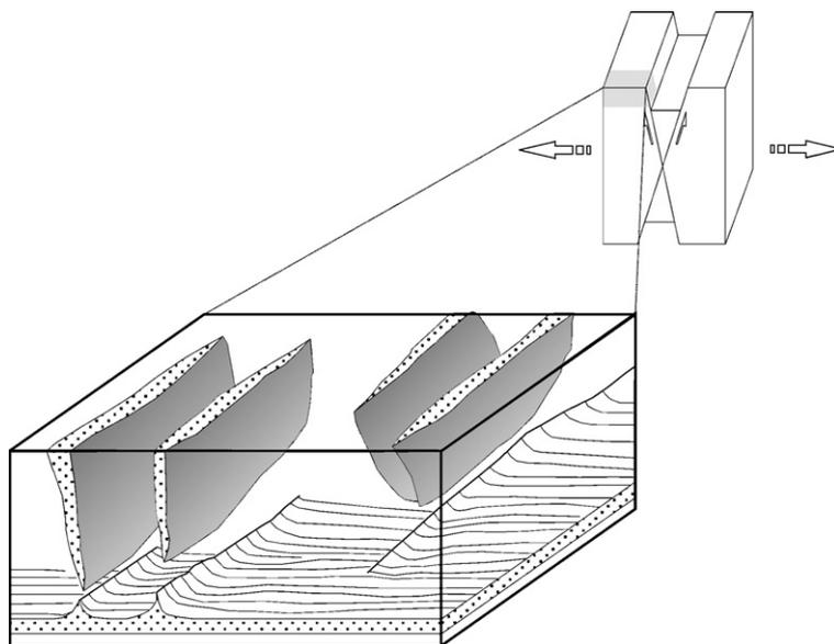
Fig. 9. Sketch of the injection of calciclastic sediments into joints and relation to the syn-sedimentary normal faults.
