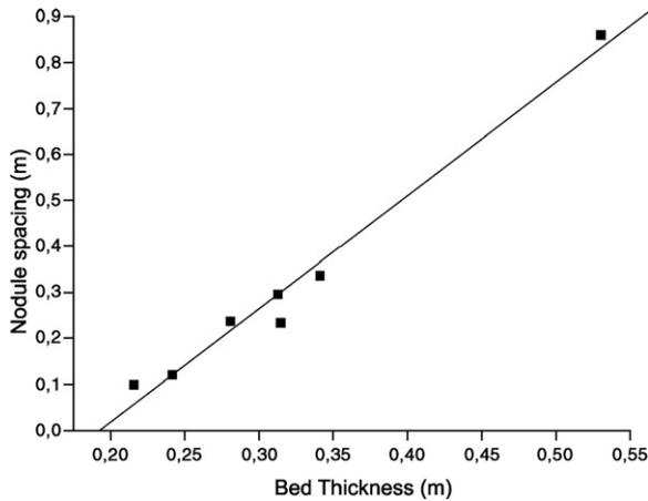
Fig. 8. Scatter plot of the fine-grained carbonate average bed thicknesses *versus* the average spacing of the hosted chert nodules. The observable linear correlation suggests the occurrence of calciclastic sediments injection along joints (see text for discussion).
